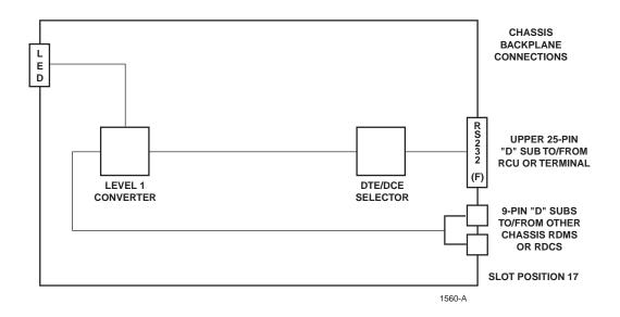
Figure 2-14. PSR-06 Interface Converter
